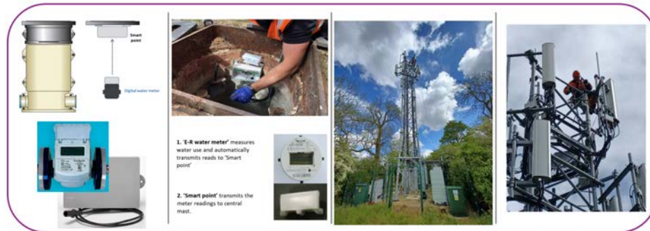
Figure 25 Smart meter technologies - trialling
